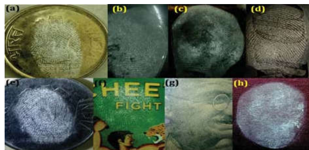
Fig. 3: Alumina-developed fingerprints on porous/textured/engraved surfaces (a) a nickel brass (German silver) currency coin, (b) a black color plastic mouse, (c) a SS lock, (d) engraved area of a CD, (e) a SS currency coin, (f) a multicolored match box, (g) a currency paper, and (h) a jewellery cloth box.
