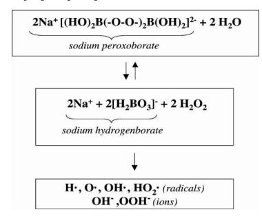
Figure: After adding water to sodium peroxoborate,  $H_2O_2$  is formed that is further decomposed into different radicals or ions.
