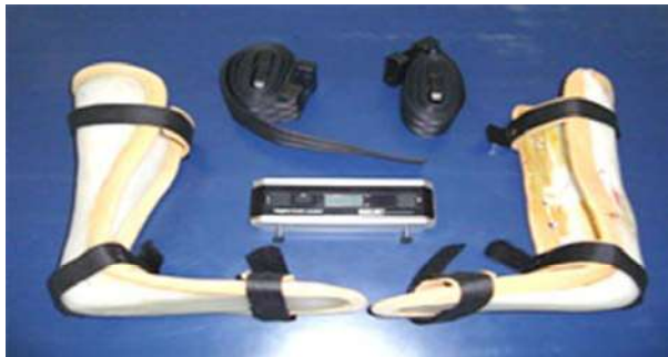
Mulligan belt, digital inclinometer and ankle foot orthoses
